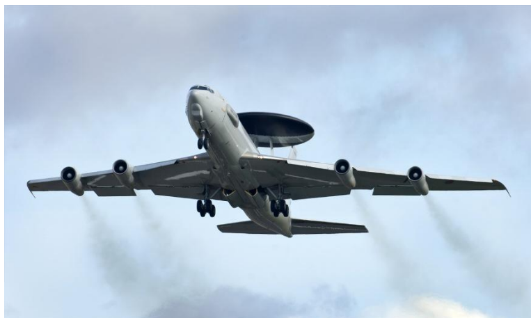
Figure 5: AWACS reconnaissance aircraft primarily use microwave radar technologies for air surveillance, target tracking and early warning
